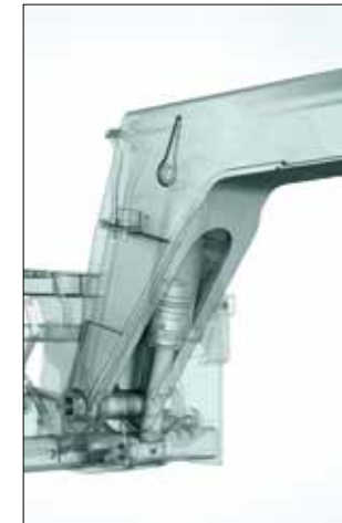
Integrated nose and one-piece closing plate
